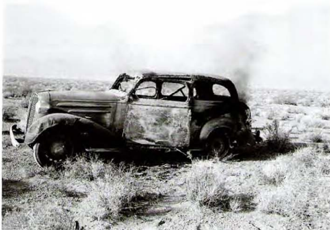
Chevrolet two-door sedan placed one-and-a-half miles from ground zero still burning four hours after the shot. Oriented at about 60 degrees from the blast, the car was completely burned. The glass was destroyed as a result of the fire. The headlights were not broken, and the chrome was not charred. The top was warped. The front tires remained inflated and intact. Source: Los Alamos National Laboratory.
